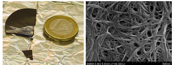
FIG. 7: Left: image of single-wall carbon nanotube paper on aluminum foil, compared in size to a one euro coin. Right: Scanning electron microscopy image of the same nanotube paper.
